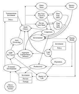
Figure 3. CLIOS Diagram for Mexico City Transportation Subsystem
